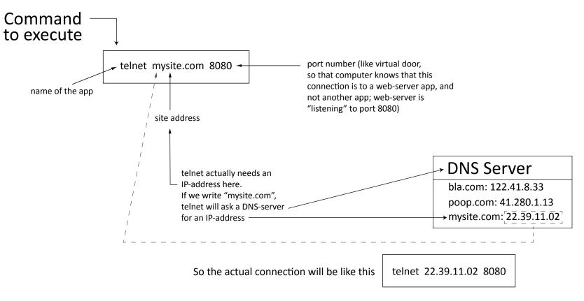
After telnet connection is established, you can type the HTTP request
